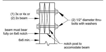
Figure 9: Prohibited Post-to-Beam Attachment Condition
