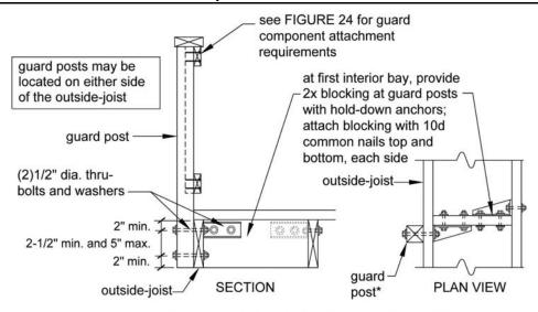
\*guard posts can be installed as shown in Figure 26 (between joists) if blocking is installed as shown above within 12" of each side of the post
