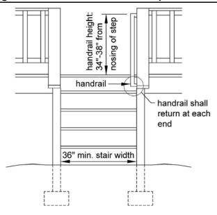
Figure 34: Stair Footing Detail
