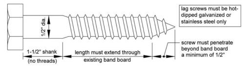
**Lag screw installation requirements:** Each lag screw shall have pilot holes drilled as follows: 1) Drill a ½" diameter hole in the ledger board, 2) Drill a  $^5/_{16}$ " diameter hole into the band board of the existing house. DO NOT DRILL A ½" DIAMETER HOLE INTO THE BAND BOARD.
