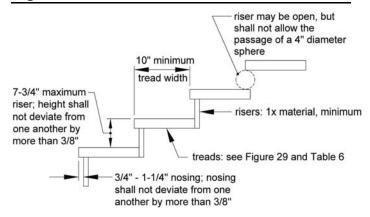
**Figure 29: Tread Connection Requirements**
