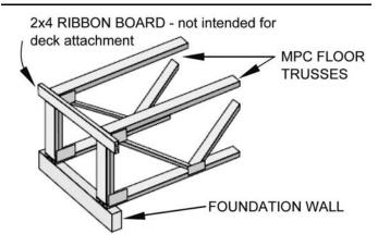
Figure 14: General Attachment of Ledger Board to Band Joist or Rim Board
